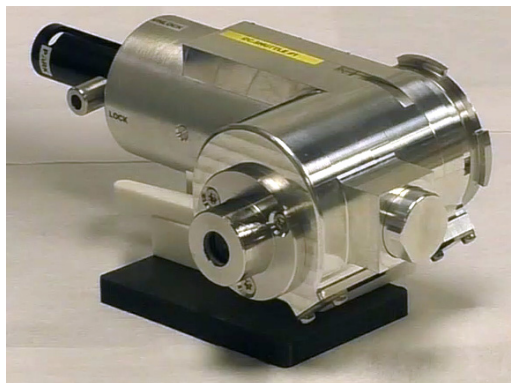
FIGURE 7-13 CC Shuttle (the pressure gauge is not present)
