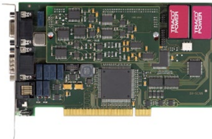
Fig. 3.1-2 PCI-plug in IO-Scan
